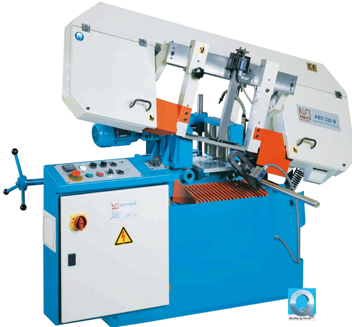
A bundle vise is provided for cutting entire material packs to length
